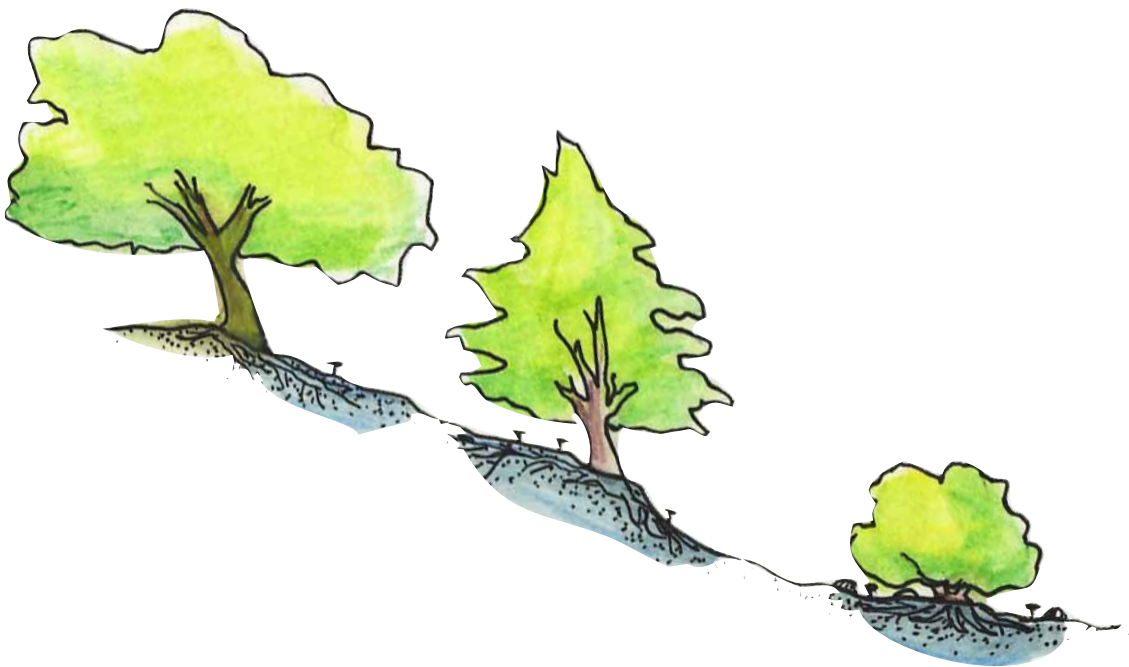
FIGURE 4: The tree on the left will be subject to wind damage and poor growth due to improper emitter placement and restricted root growth. The middle tree illustrates proper emitter placement for slope plantings. The shrub on the right uses a watering basin, or berm, to hold water near the root zone.
